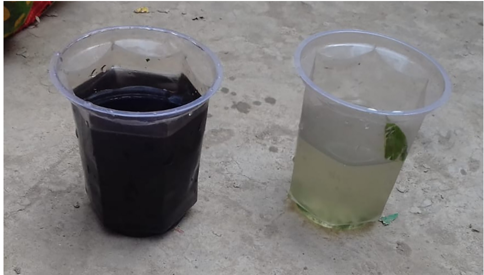
Fig 2. Treated water demonstration—Drinking water 2-minutes after crushed guava leaves are added to untreated ground water (left) versus treated ground water (right).
