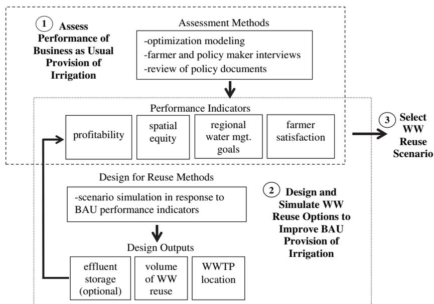
**Fig. 1 – Overview of methods and performance indicators comprising the coupled performance assessment and optimization model for designing wastewater treatment systems for reuse in agriculture. The three-step planning model includes (1) a performance assessment of the business as usual provision of irrigation, (2) simulation of various reuse scenarios, and (3) selection of a reuse scheme based on the comparative performance of the reuse scenarios to the baseline performance.**
